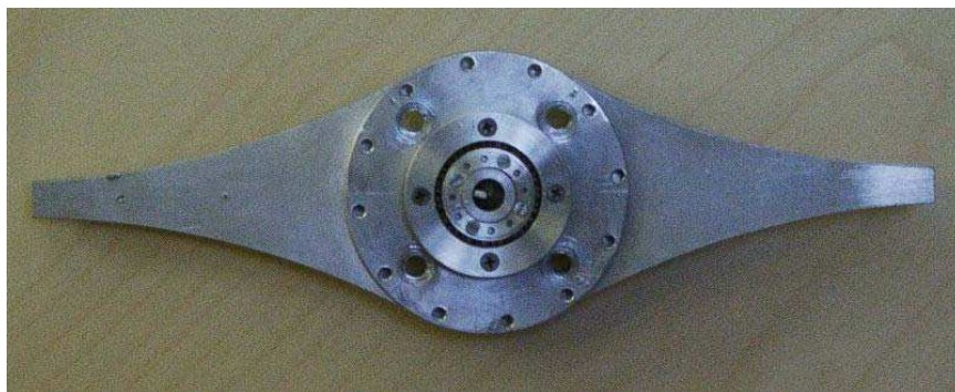
Fig.2. Photo of the accelerating arm of ITV5.1 centrifuge pellet injector.
